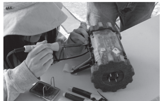
Fig.3 Attaching Resistances for Removing Parachute
