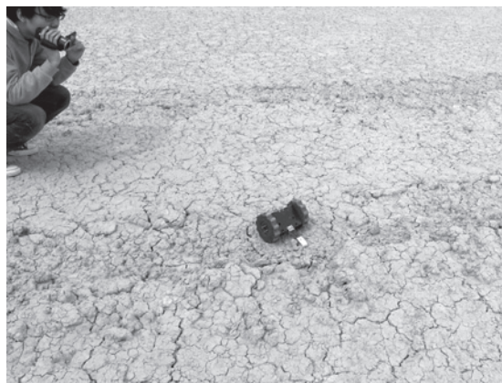
Fig.8 Rover Stucked in a Rut
