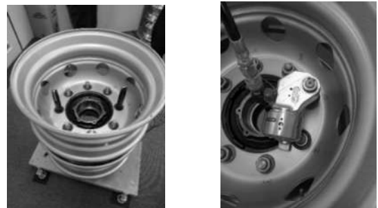
(c) An outer wheel guided by two proper jigs (left hand side figure) (d) Wheel nuts tightened by oil pressure wrench
