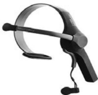
Fig.1 Electroencephalograph(Mindwave Mobile2)<sup>[3]</sup>
